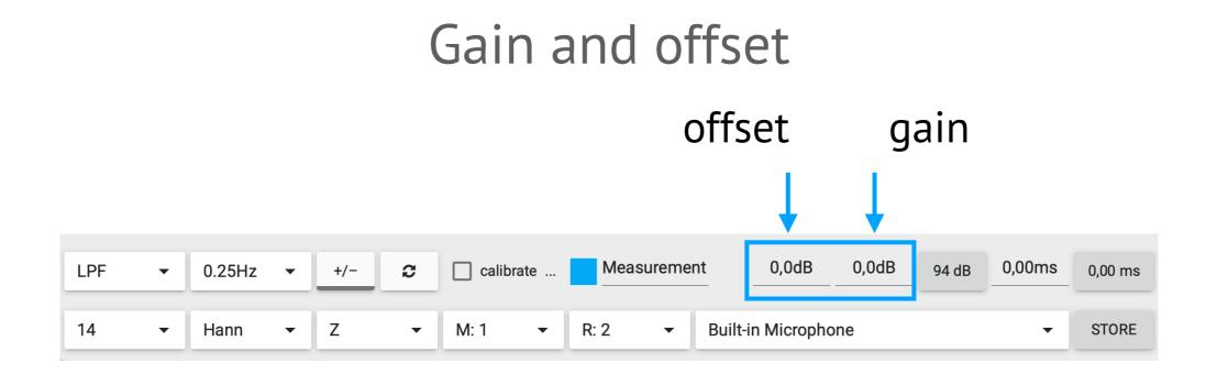
Offset - offset for 0 at magnitude response (gain for reference channel)
