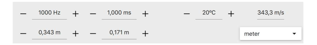
Allows you calculate between frequency, period and wavelength. You can change any value and get others. Use Shift key to fine adjust value
