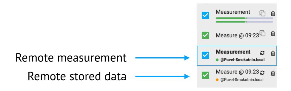
Remote sources shown in the side bar as a regular sources with a label from what host it was taken. Each remote source has coloured label:
